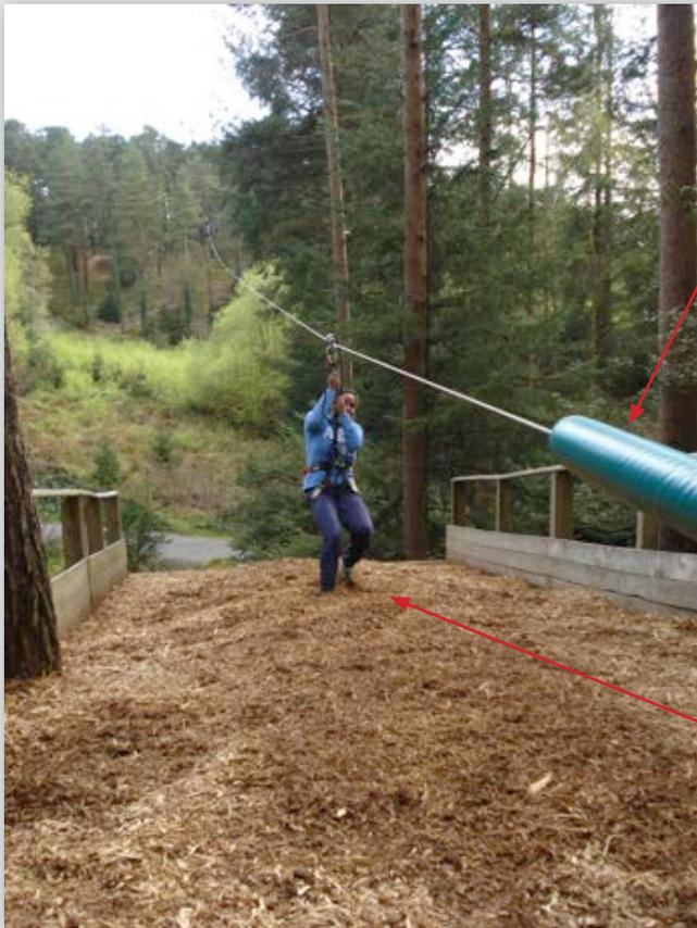
Emergency brake (e.g. spring covered by foam) must be passive
